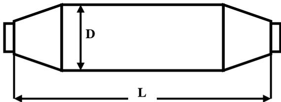
The diagram shows a side view of a catalytic converter. It has a central cylindrical section with a diameter labeled 'D' and a total length labeled 'L'. Both ends of the converter are tapered into conical shapes.
