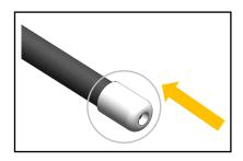
7. Pull the bovden cable through the gear lever. **Be careful not to let the cable end cap fall out.** Then insert the bovden cable into the hole of the locking lever. **Push forcefully on the bovden so that it is inserted as far as possible, at the same time tighten the set screw on the locking lever**. For this use tools from zip bag **4**.
