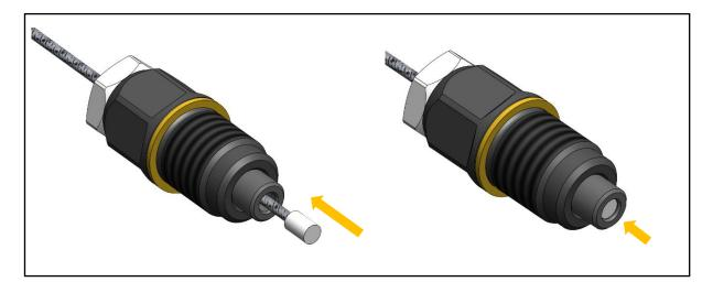
5. Then dimple the head of metal cable to prevent it from falling out.
