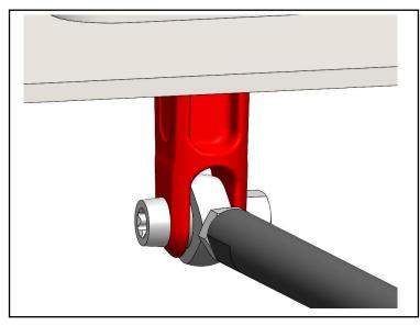
3. Unscrew the gear lever head (black part). Turn counterclockwise. Perform the operation by hand without any tools to prevent damage to the head.
