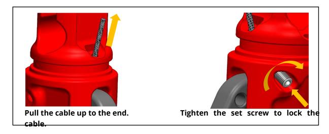
To verify proper installation, try to check that the locking lever does allow 1-2 mm free movement, as well as the end of the bovden cable on the gearbox lock flange. Repeat step 6 if any of these problems occurs (LITTLE FREE MOVEMENT, 1-2mm is REQUIRED).
